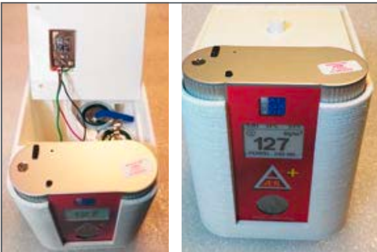
Fig. 1 | Radon housing with power supply. On the left the small power supply PCB.
