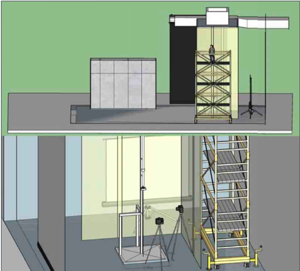
Fig. 1 | Schematic representation of the Ash-Burster, designed to study volcanic particle aerodynamics in a large spatial domain.
