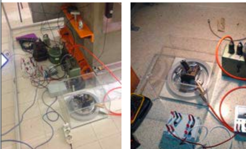
Fig. 2 | Experimental installation of the rotational sts-1 near GINGER (left) and in Rocca di Papa museum basement (right).
