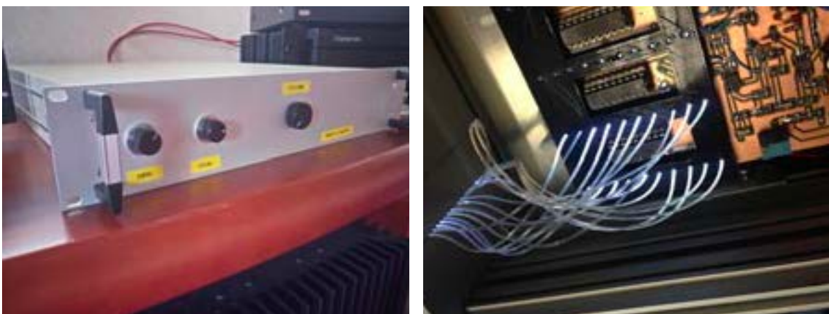
Fig. 1 | The last prototype of the audio amplifier (left). The first knob allows the use to tune the loudspeaker damping factor. On the right a particular of the vu-meter.
