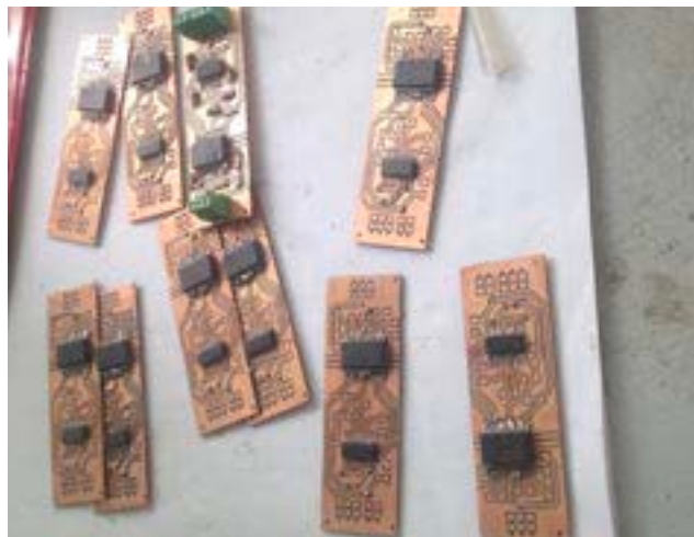
Fig. 2 | Galvanically isolated serial interfaces have been widely used to allow electrically safe connections between sections of the gondola electronics.
