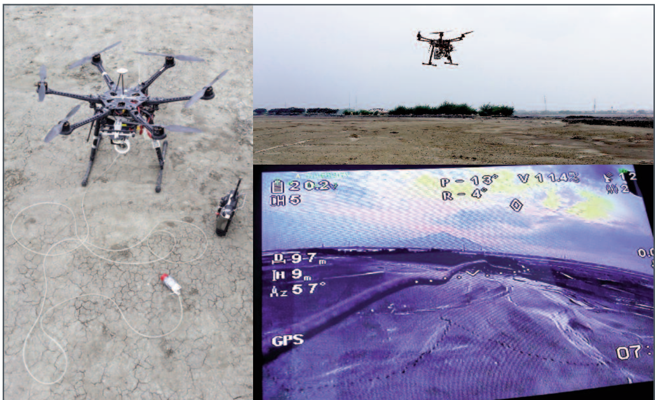
Fig. 1 On the left the drone, equipped with the gas sensor developed by La Sapienza, connected with a 5m long pipe and a filter. On the right, up, the drone flies carrying both the INGV's and Sapienza's gases sensors. On the right, bottom, the screen of the fpv monitor during a flight.
