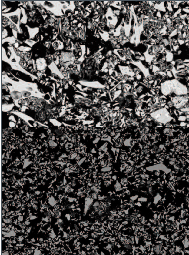
Fig. 1 | Back scattered electron (BSE) images showing some of the studied tephra sampled in Patagonia (Chile).
