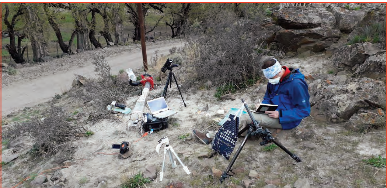
Fig. 1 | Deploying the portable wind tunnel in Argentina (October 2019), to study the resuspension of volcanic ash deposited from Cordon Caulle 2011 (Chile) eruption.
