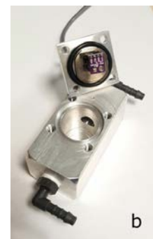
Fig. 11. (a) Acquisition board based on RaspberryPi and BME280 chip-sensor which measures air parameters: RH, pressure, temperature. (b) BME280 sealed housing, employed for pipe in-line insertion of the device.
