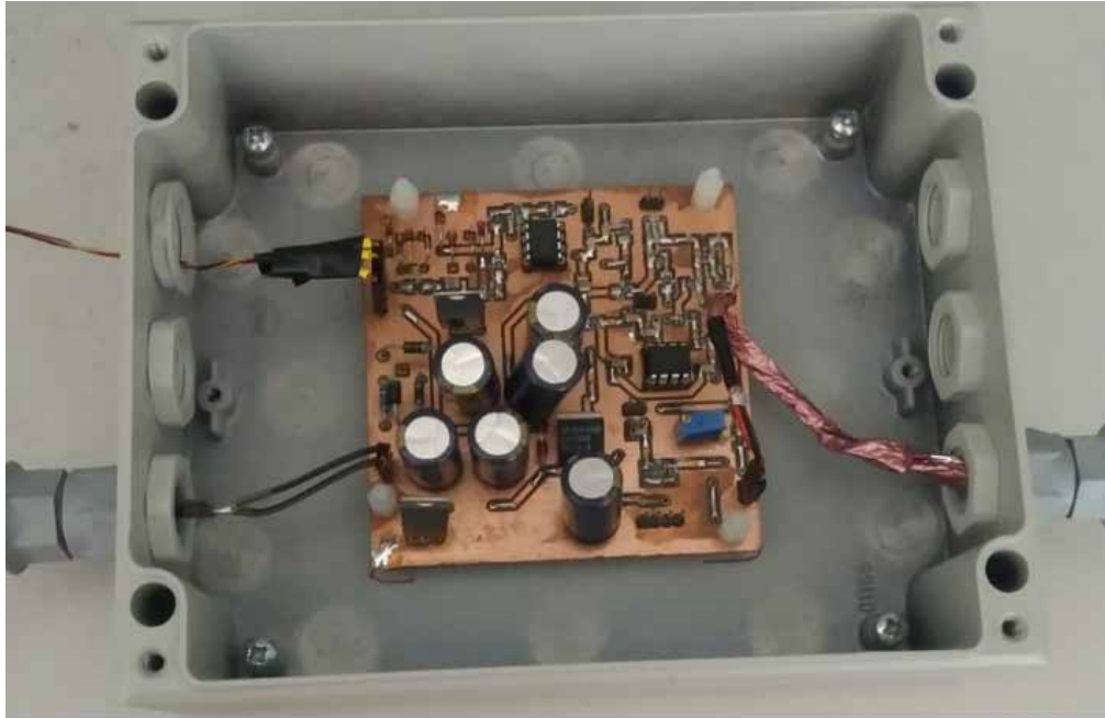
Fig. 1| Filter inside the metallic Box.
