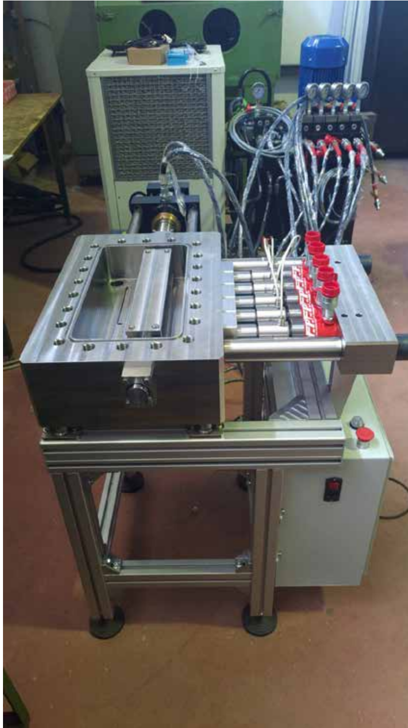
Fig. 11 The novel biaxial apparatus MEERA, MEchanics of Earthquake and Extended Rupture Apparatus recently installed in the HPHT laboratory of the INGV.
